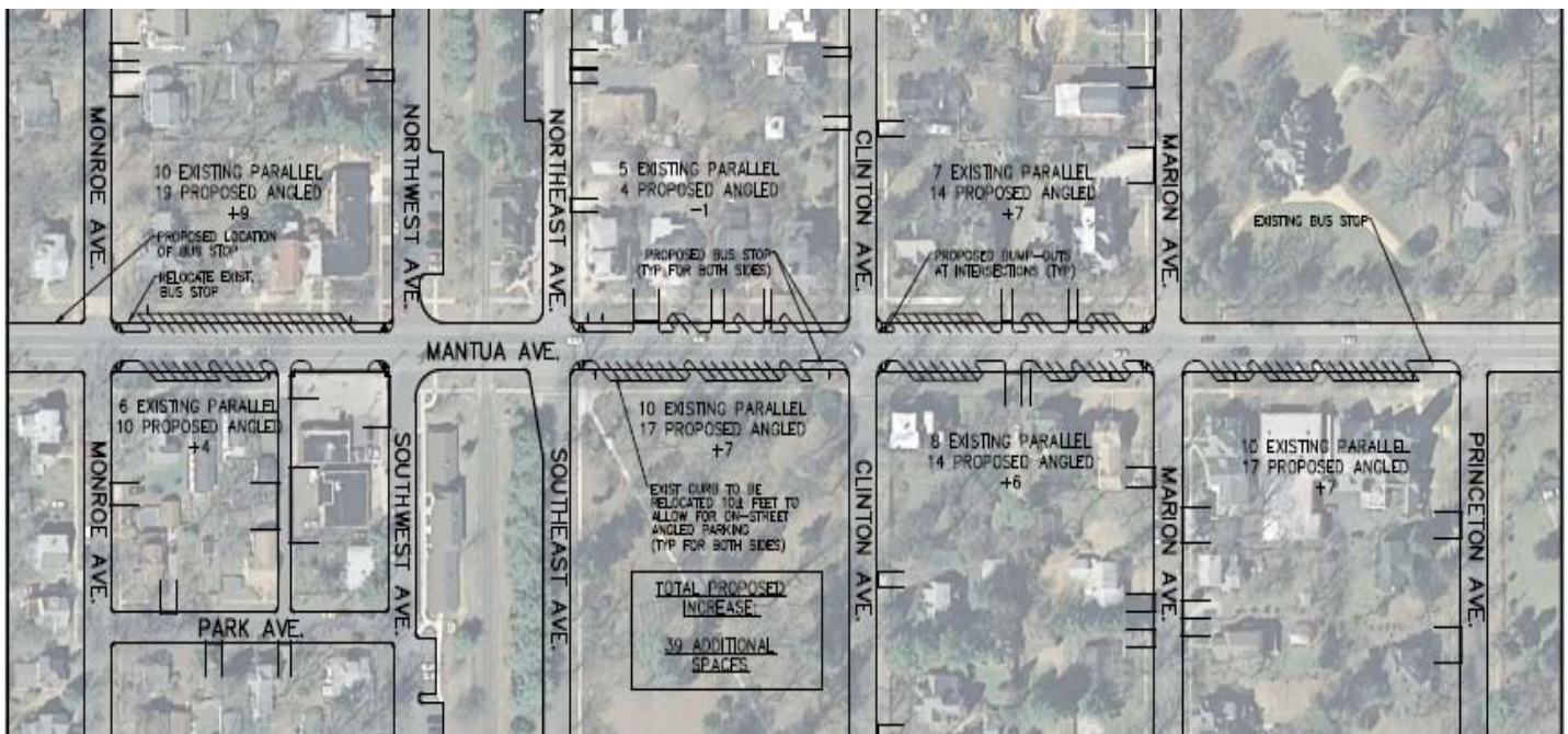
FIGURE 10: ANGLED PARKING IMPROVEMENTS IN MANTUA AVENUE
