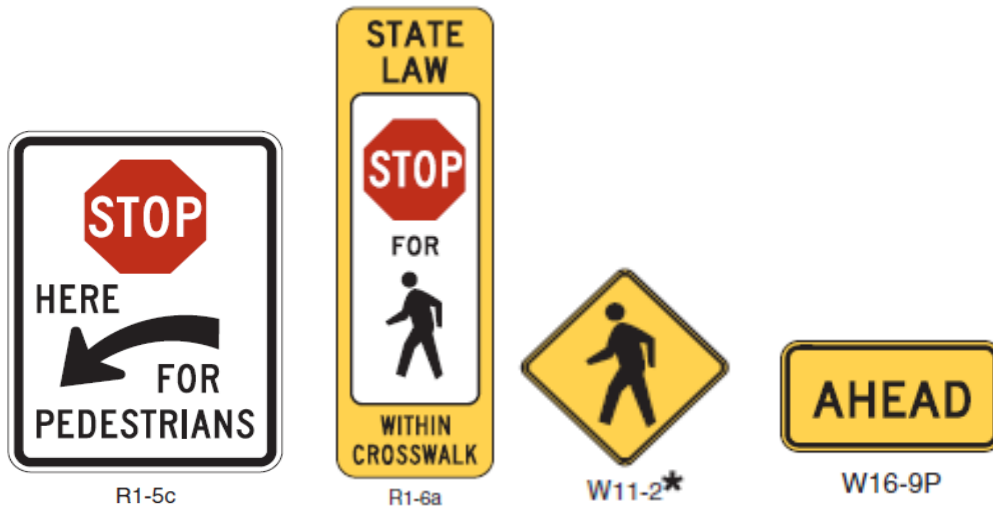
FIGURE 17: PEDESTRIAN ROAD CROSSING SIGNAGE
